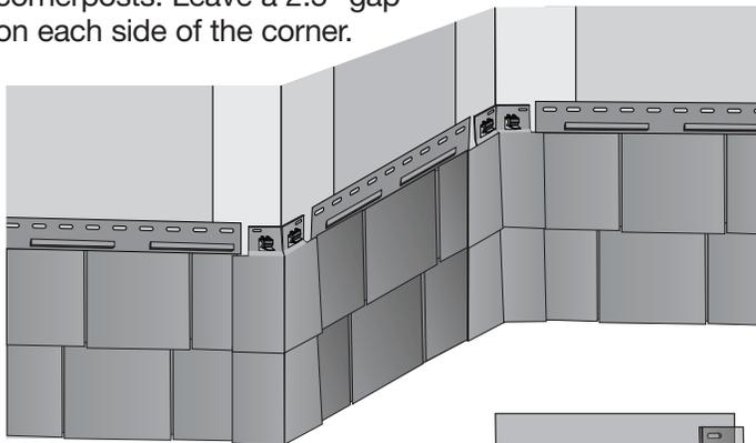
4. Once the panel has been fastened, hook the cornerposts over the siding, making sure they are locked into the starter strip.
