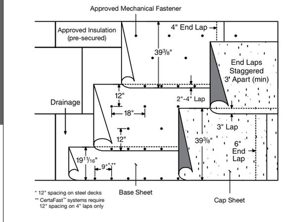
**Base sheet mechanically attached through insulated substrate and an SBS modified cap sheet**
