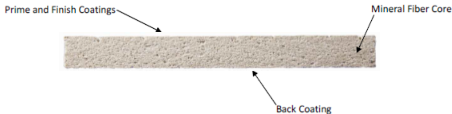
Figure 3: Diagram of Protectone Product Family Construction
