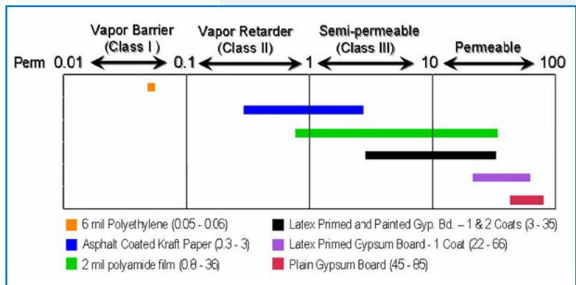
**Figure 3.** The above chart shows where the most common vapor retarder materials stand in the most current vapor retarder permeance rating system established by the 2007 supplement to the 2006 International Residential Code.
