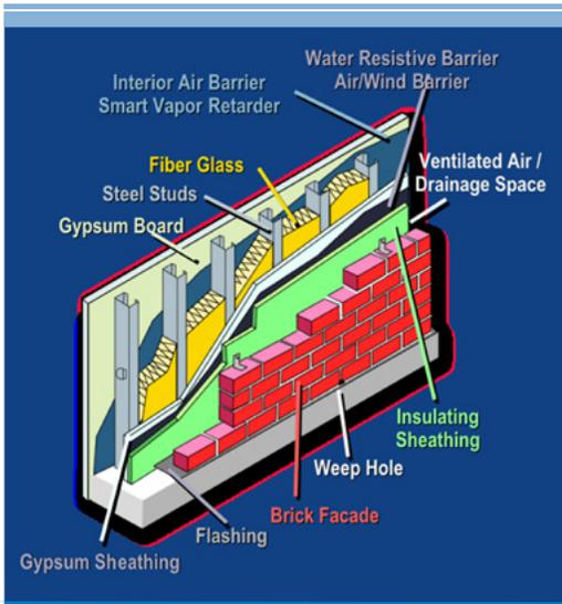
The steel stud cavity assembly is the most common commercial wall construction. For the best moisture management performance, such assemblies should always consist of a water-resistant barrier, insulating sheathings, exterior air/wind barriers, interior air barriers and a smart vapor retarder to not only control the wintertime moisture but also to allow assemblies to breathe during other seasons.
