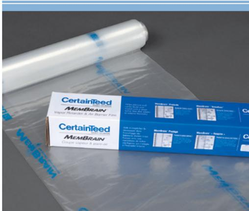
MemBrain™ is a smart vapor retarder that changes its permeability to water vapor as ambient humidity changes.
