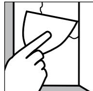
Next, fold the tape and lightly press it into the corner with your knife.
