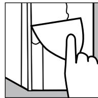
Using even pressure, press paper / metal bead onto corner into position, ensuring it is aligned; embed it into compound by running the knife at 45° angle. Let dry for 24-hours. Apply a second coat with the 7"
