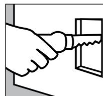
For larger openings, install the panels directly across the openings. Then use a drywall saw to cut the panels, using the framing as your guide. As you install the boards, make sure that you do not place joints at the edges of doors or windows. If you do, as the door or window is opened and closed over time, the joint will crack.
