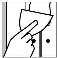
First, apply a coat of Easi-Fil® joint compound over the joint with your four-inch knife. Then, press the tape firmly into the compound by pressing your knife over the tape. Squeeze out excess compound, making sure
