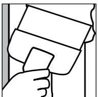
Apply a third coat using a 12" tapping knife and this coat should be a thin coat and should extend approximately 7-12" beyond each side of the joint. The further you feather the compound out, the harder it will be to see imperfections.
