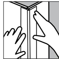
Measure bead and cut to right length; a snug fit from floor to ceiling (about 1/4" shorter than the wall height). With a 7" knife apply a generous amount of Easi-Fil joint compound on either side of corner.
