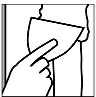
Apply a second coat using a 7" tapping knife and this coat should extend approximately 4" - 6" beyond each side of the joint. After the coat dries approximately 24 hours, sand the area
