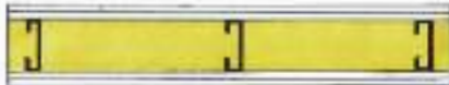
Rating: 2-hour non-bearing (U 420) Chase wall: Double layer 5/8" Type X gypsum board on each side 1 5/8" steel studs on 24" centers 2 1/2" CertainTeed fiber glass insulation
