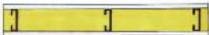
Rating: 1-hour non-bearing (U 419) Single layer 5/8" Type X gypsum board on each side Min. 3 1/2" steel studs on 24" centers 3 1/2" CertainTeed fiber glass insulation
