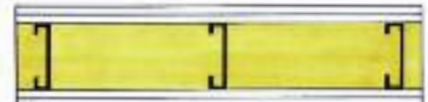
Rating: 2-hour non-bearing (U 419) Double layer 5/8" Type X gypsum board on each side 6" steel studs on 24" centers 6 1/4" CertainTeed fiber glass insulation
