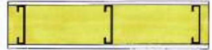
Rating: 1-hour non-bearing (U 465 or U 419) Single layer 5/8" Type X gypsum board on each side 6" steel studs on 24" centers 6 1/4" CertainTeed fiber glass insulation
