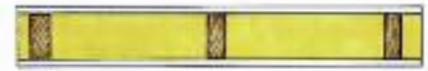
Rating: 3/4-hour bearing (U 317) Single layer 1/2" Type X gypsum board on each side 2" x 4" wood studs on 16" centers 3 1/2" CertainTeed fiber glass insulation
