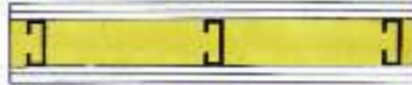
Rating: 2-hour non-bearing (U 411 or U 419) Double layer 5/8" Type X gypsum board on each side 3 5/8" steel studs on 24" centers 3 1/2" CertainTeed fiber glass insulation
