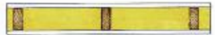
Rating: 1-hour bearing (U 305) Single layer 5/8" Type X gypsum board on each side 2" x 4" wood studs on 16" centers 3 1/2" CertainTeed fiber glass insulation
