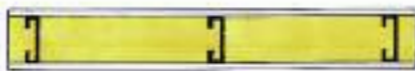
Rating: 1-hour non-bearing (U 419) Single layer 5/8" Type X gypsum board on each side Min. 3 1/2" steel studs on 24" centers 3 1/2" CertainTeed fiber glass insulation
