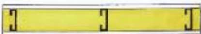
Rating 1-hour non-bearing (U 465) Single layer 5/8" Type X gypsum board on each side 3 5/8" steel studs on 24" centers 3 1/2" CertainTeed fiber glass insulation
