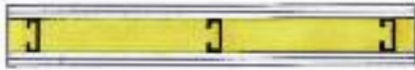
Rating: 2-hour non-bearing (U 419) Double layer 1/2" Type X gypsum board on each side 2 1/2" steel studs on 24" centers 2 1/2" CertainTeed fiber glass insulation
