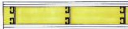
Rating: 2-hour non-bearing (U 436) Chase wall: Double layer 5/8" Type X gypsum board on each side 1 5/8" steel studs on 24" centers CertainTeed fiber glass insulation to fill cavity
