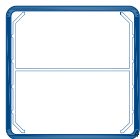
SECTION A-A LINE POST STIFFENER ALUMINUM INSERT
