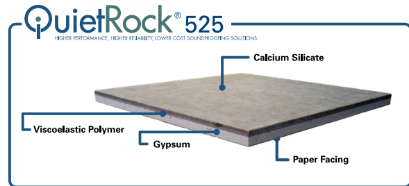
QuietRock is a multi-layer engineered drywall panel made of gypsum and viscoelastic sound absorbing polymers.
